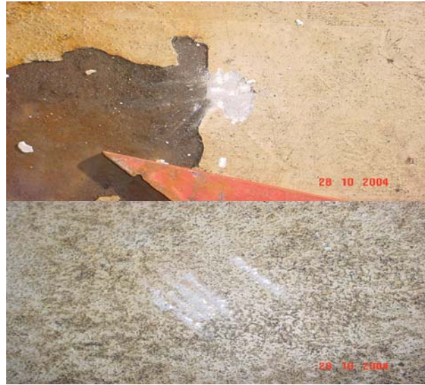
Figure 7 This is part of a destructive test for traffic decks on a RoRo subjected to extreme loads of 120 ton containers. The upper slide illustrates a ceramic pigmented epoxy coating and the lower in an MCU zinc and aluminium system.
