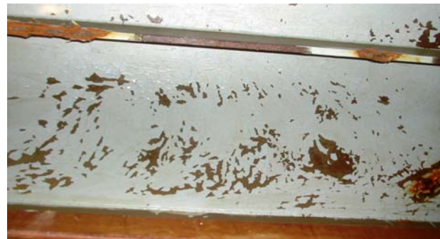
Figure 2 This paint cracking caused by hull flexing (likely a reverse impact) and a coating choice that was too rigid. The top coating adhesion was not good and when the membrane broke the result is intercoat adhesion failure causing the paint to peel. A contributing factor to this could be that the surface was either damp when coated or the surface may have reached the dew point before it had a chance to cure.
